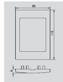
*\*Painting of different colours shall be made by the customer: in this case order the unassembled version of the article. For the installation is required a standard 503 flush mounting box (not provided).*
